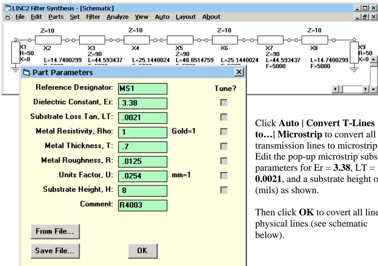
Click **Auto | Convert T-Lines to... | Microstrip** to convert all transmission lines to microstrip. Edit the pop-up microstrip substrate parameters for  $E_r = 3.38$ ,  $LT = 0.0021$ , and a substrate height of **8** (mils) as shown.
