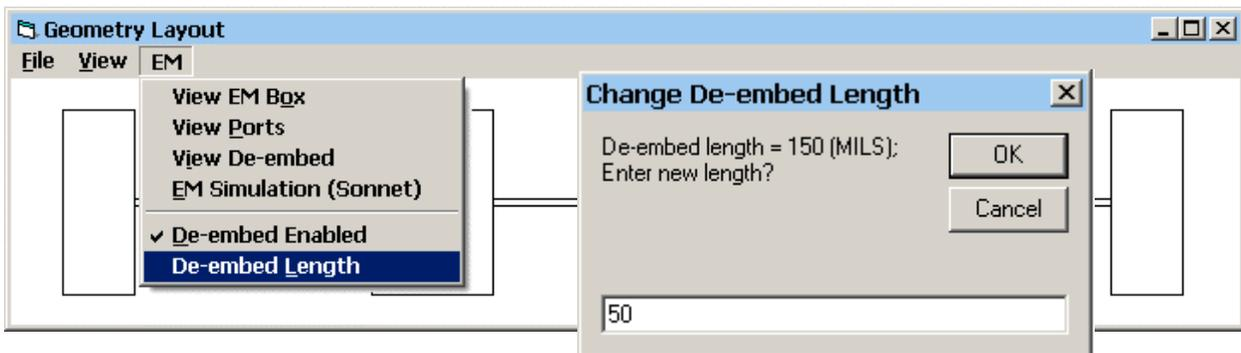
When EM Simulation (Sonnet) is selected, the file EMTTest.SON is created and automatically exported to the Sonnet<sup>®</sup> xgeom project editor ready for analysis. The EM box, metal and substrate layers and frequency parameters are already loaded. The layout in Sonnet<sup>®</sup> is shown below. Black arrows pointing inward from each port show the amount of de-embedding at the ports.
