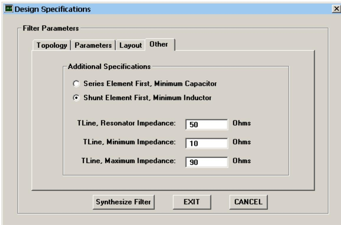
Click the **Other** tab. Select **Shunt Element First** and change the TLine (transmission line) minimum and maximum impedances to 10 and 90 ohms respectively. The filter specifications are now complete. Click the **Synthesize Filter** button and **Exit** to see the filter schematic (below).
