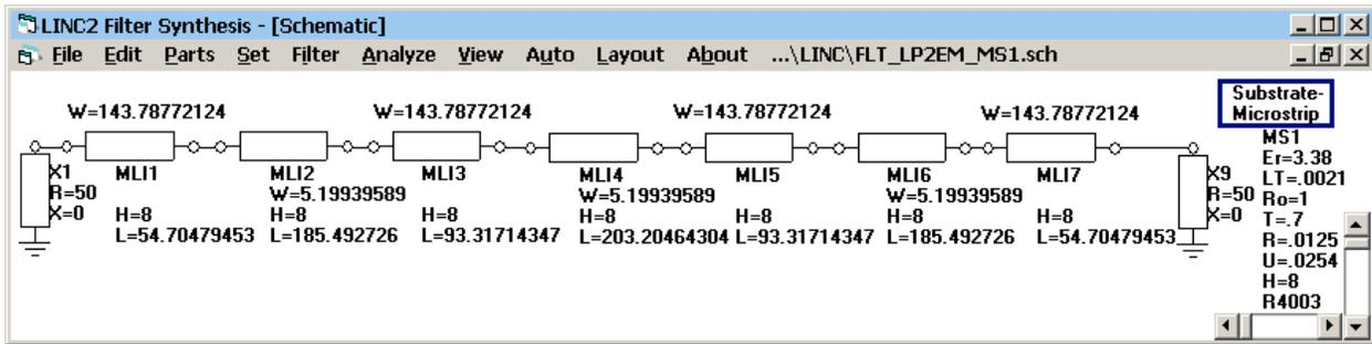
The resulting schematic is converted to all physical microstrip lines. Click **Layout** to see the layout geometry (below).
