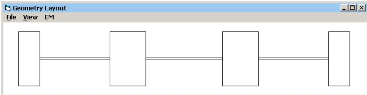
For this example, change the default de-embedding length from 150 mils to 50 mils by selecting **De-embed Length** from the EM menu as shown below. Enter 50 and click OK. Then select **EM Simulation (Sonnet)** from the EM menu.
