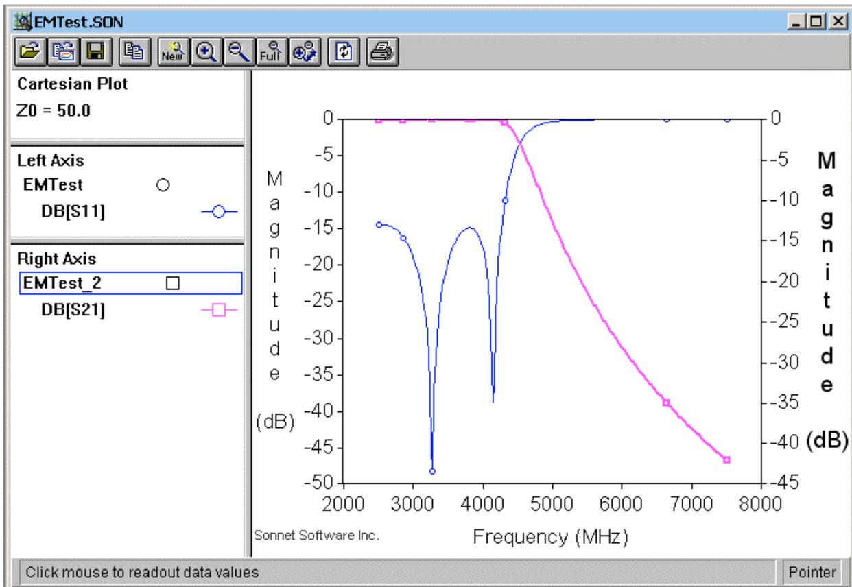
The plot of S21 shows that the filter response is lowpass with a cutoff frequency slightly ahead of the 5000 MHz design goal. The return loss (S11\_dB) in the passband is 15 dB or greater.
