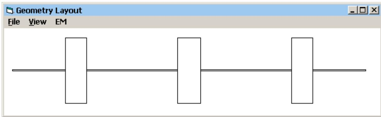
For this example, remove the de-embedding option by un-checking **De-embed Enabled** from the EM menu as shown below. Then select **EM Simulation (Sonnet)** from the EM menu.
