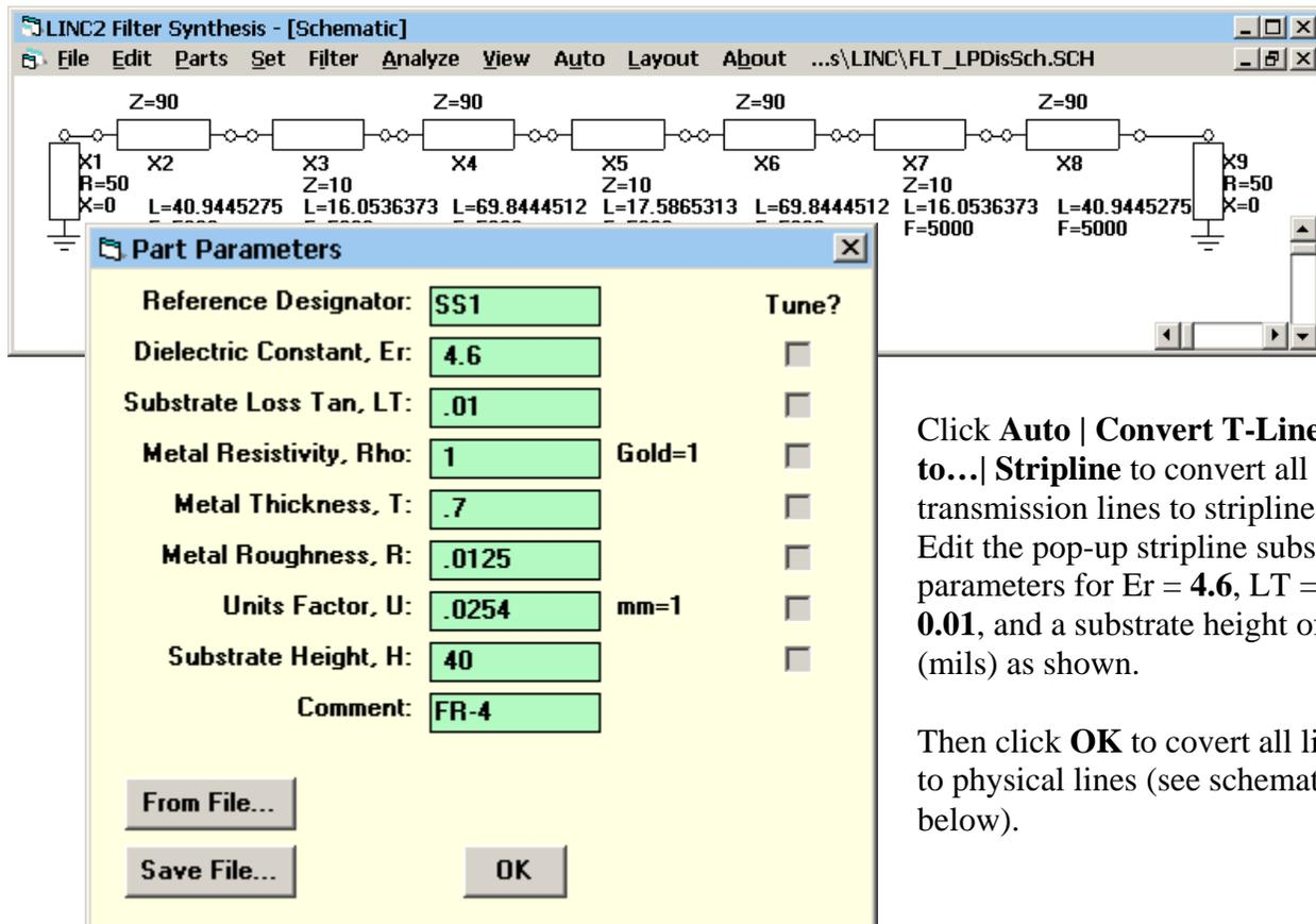
Click **Auto | Convert T-Lines to... | Stripline** to convert all transmission lines to striplines. Edit the pop-up stripline substrate parameters for  $Er = 4.6$ ,  $LT = 0.01$ , and a substrate height of **40** (mils) as shown.
