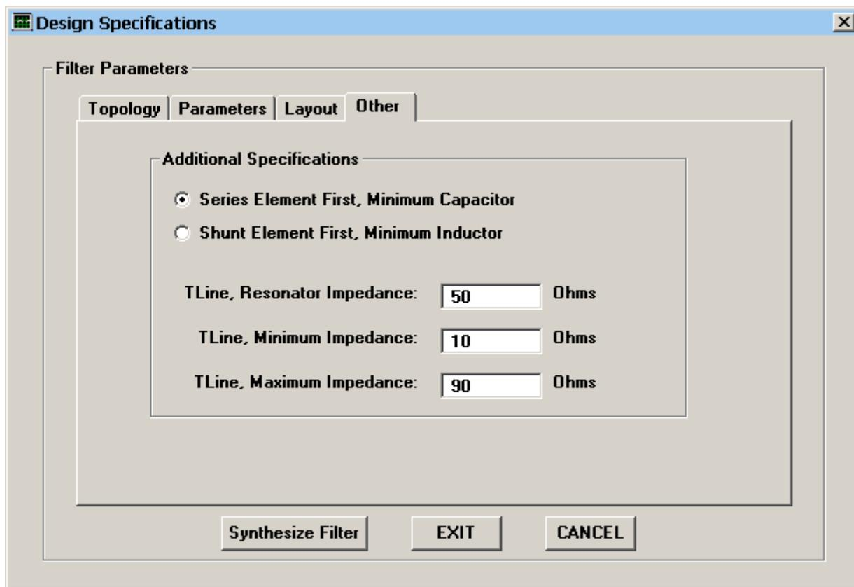
Click the **Other** tab and change the TLine (transmission line) minimum and maximum impedances to 10 and 90 ohms respectively. The filter specifications are now complete. Click the **Synthesize Filter** button and **Exit** to see the filter schematic (below).
