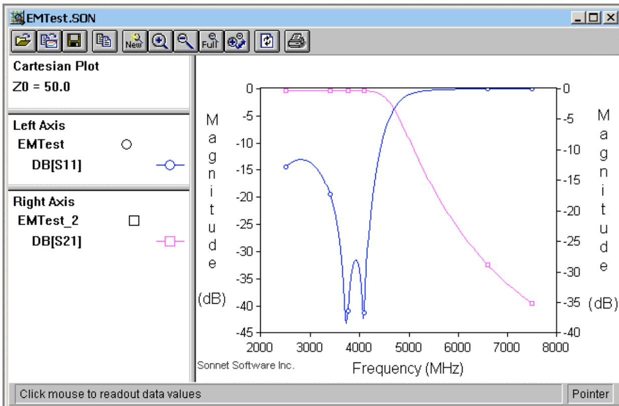
The plot of S21 shows that the filter response is lowpass with a cutoff frequency slightly ahead of the 5000 MHz design goal. The insertion loss in the passband ranges between 0.3 and 0.4 dB, which is very close to the 0.15 dB passband ripple specified.
