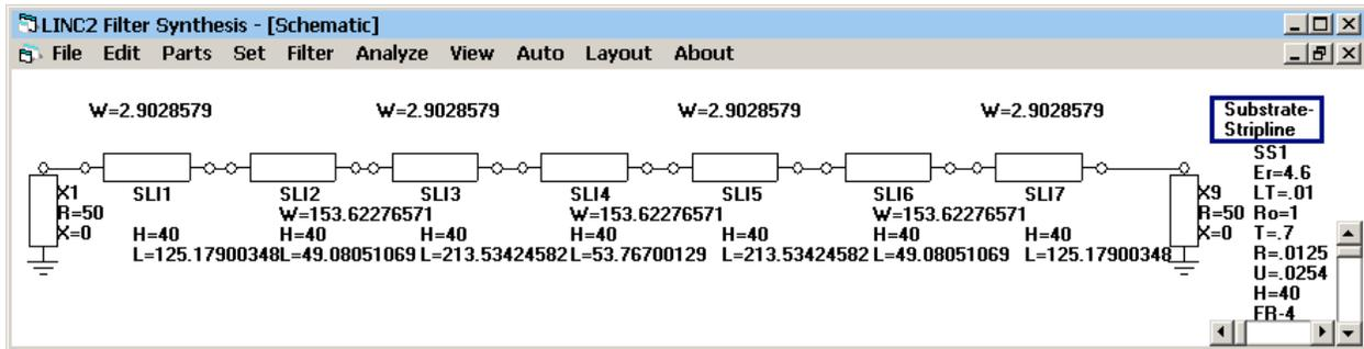
The resulting schematic is converted to all physical T-lines. Click **Layout** to see the layout geometry (below).
