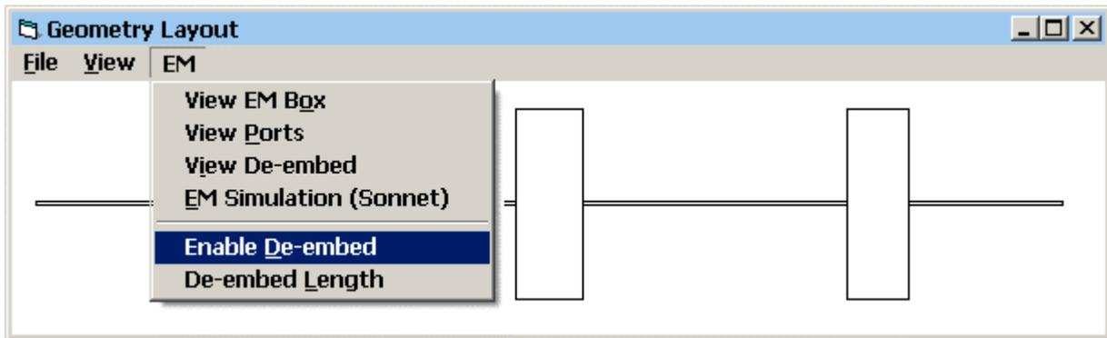
When EM Simulation (Sonnet) is selected, the file EMTTest.SON is created and automatically exported to the Sonnet<sup>®</sup> xgeom project editor ready for analysis. The EM box, metal and substrate layers and frequency parameters are already loaded. The layout in Sonnet<sup>®</sup> is shown below.
