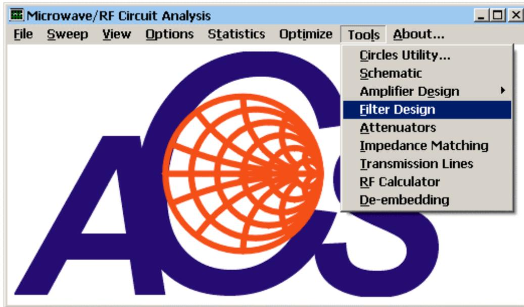
The LINC2 filter synthesis program is started by selecting **Filter Design** from the main LINC2 **Tools** menu as shown above.
