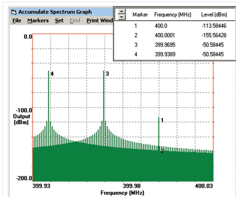
Figure 10: Spectrum Showing Phase Noise from Reciprocal Mixing Prior to IF Filtering (High Quality LO has Low Phase Noise)
