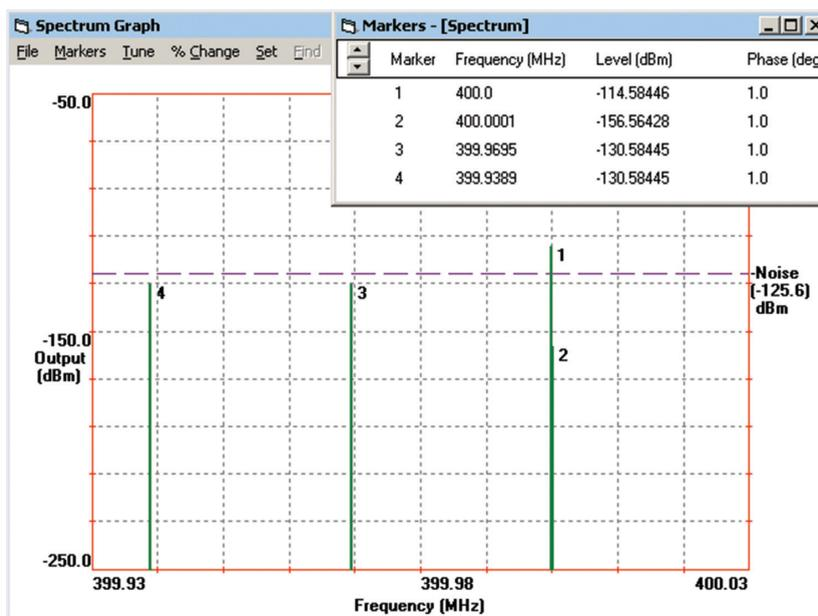
Figure 3: 400 MHz IF Spectrum with Interferers
