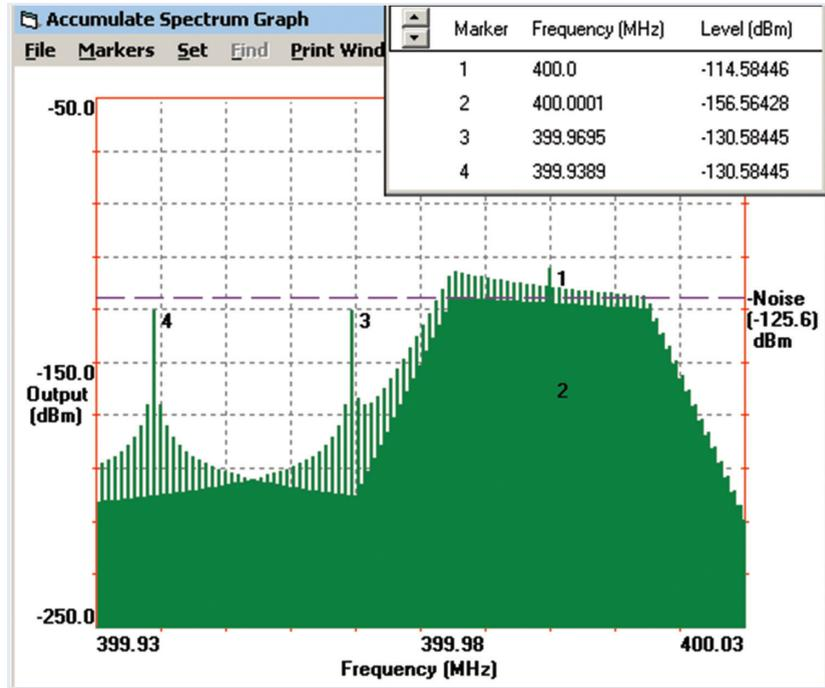
Figure 7: Spectrum Plot of Reciprocal Mixing into the IF band
