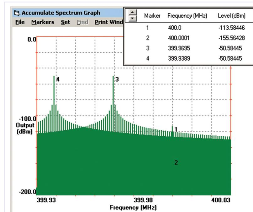
Figure 9: Spectrum Showing Phase Noise from Reciprocal Mixing Prior to IF Filtering (LO has High Phase Noise)
