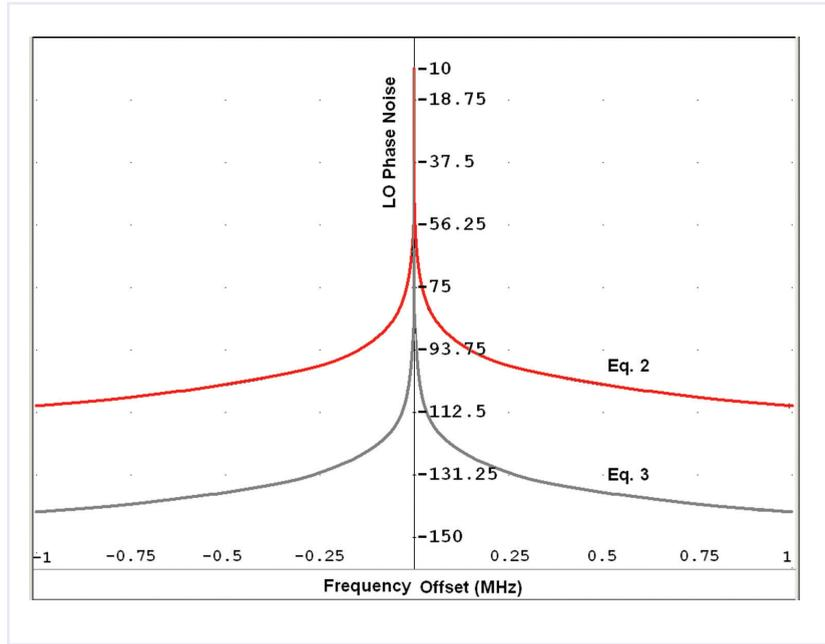
Figure 5: Double Side-Band LO Phase Noise Plots
