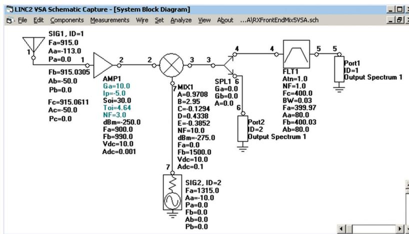
Figure 1: Receiver RF Front End (Antenna through IF)
