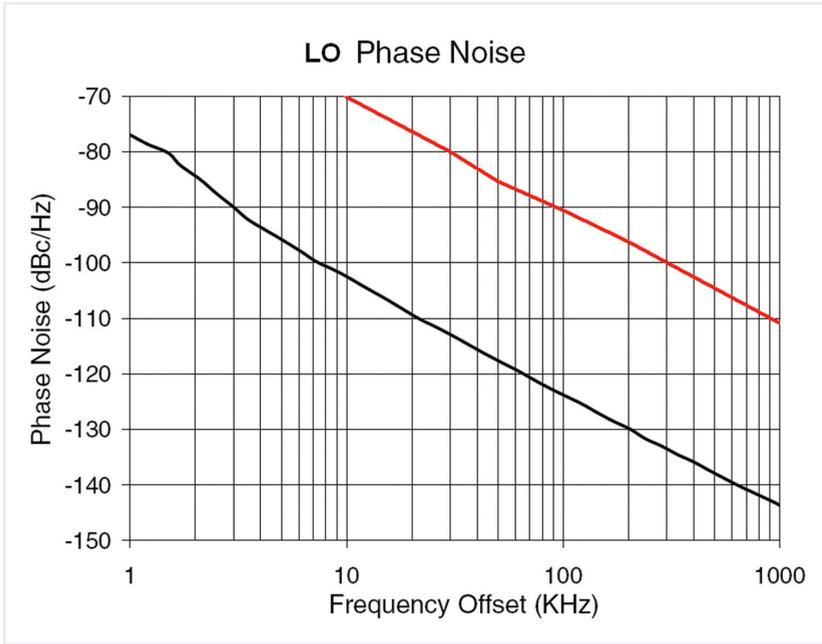
Figure 4: LO Phase Noise vs. Frequency Offset (for two different local oscillators)
